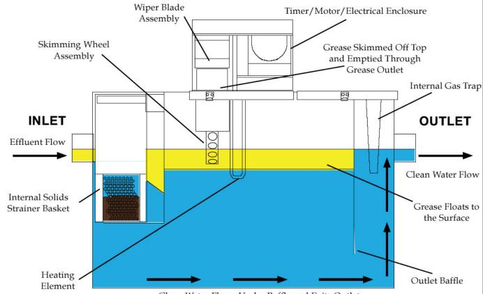
Clean Water Flows Under Baffle and Exits Outlet
