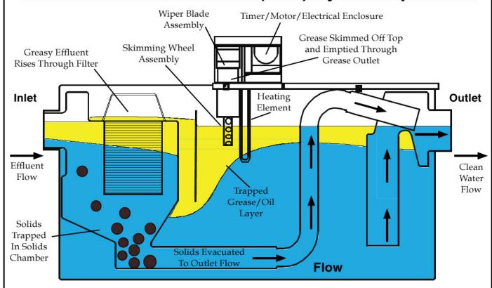
**AST** systems automatically separate and remove grease, fat, and oil from drain water flow. A patented technological breakthrough allows incidental food solids and other debris found in the effluent to be separated from the grease and pumped out of the solids retention area to the drain. The entire process is controlled automatically by a timer. The operation of the Big Dipper AST can be broken into two components.
